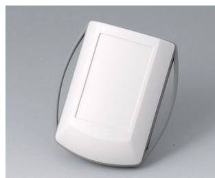
B7040227 ERGO-CASE XS ABC (UL 94 HB) белый RAL 9002 82x56x24mm IP 42
