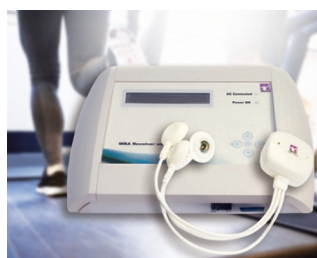
WBA receiver unit for measuring biosignals
