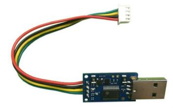
The above figure shows an M5X0-PWR board, which supplies 3.8V/0.6A power for the module and outputs 3.3 V CMOS level TXD and RXD for the communication between the computer and the module. It is connected to the N11 EVB through 4-pin cables, which have been soldered to the power board in a sequence of red, black, yellow, and green at one end and should be inserted into the plug of the EVB at the other end. There are two pins on the power board and they can control the power supply of the module.
