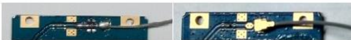
Figure 5-45 RF cable connections
