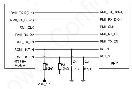
Figure 5-29 Reference design of the RMII interface
