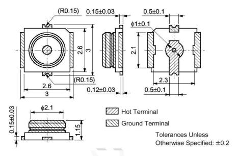
The RF cable is connected to the module by means of soldering. However, this method has the stability, consistency, and RF performance degradation issues, and therefore is not recommended.
