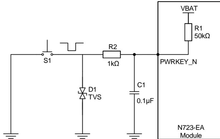
Figure 5-7 Reference design of startup, shutdown, and reset controlled by an MCU
