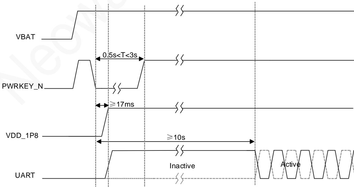
Figure 5-10 Startup process (by controlling PWRKEY)
