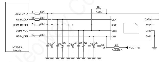
Figure 5-23 Reference design of the USIM card interface
