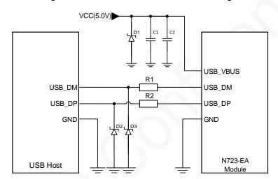
Figure 5-18 Reference USB connection design
