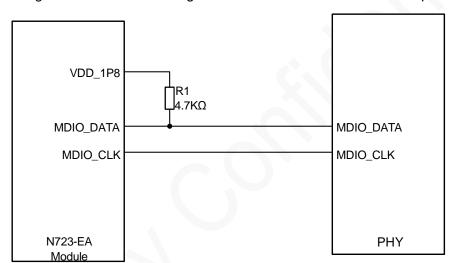
Figure 5-30 Reference design of the SDIO interface with a PHY chip:
