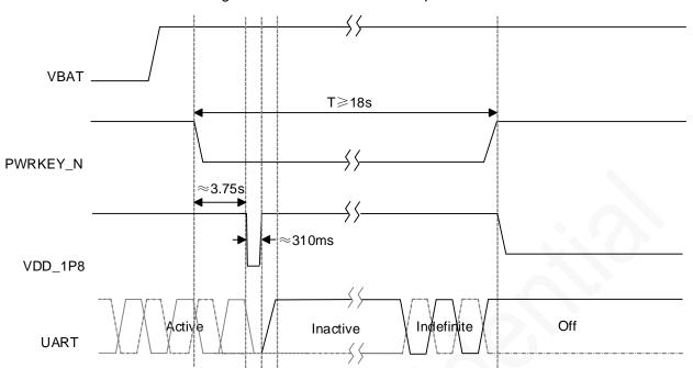
Figure 5-12 Hardware shutdown process
