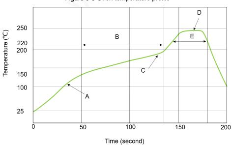
Figure 9-3 Oven temperature profile
