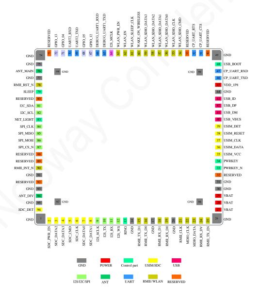
Figure 4-1 N723-EA pin definition (top view)
