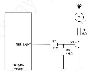
Figure 5-42 Driving LED with a triode
