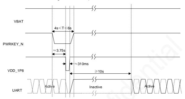
Figure 5-11 Reset process of the module
