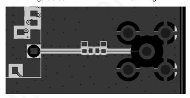
Figure 5-35 Recommended RF PCB design
