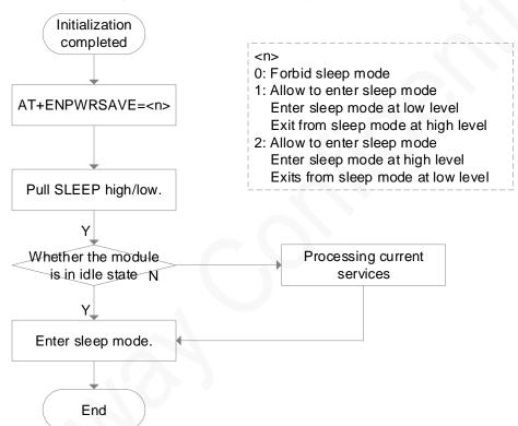
Figure 5-14 Process of entering the sleep mode
