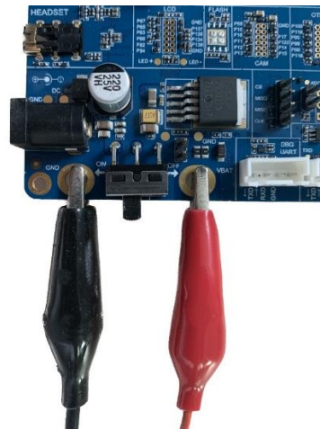
Figure 2-2 Directly connect the power supply test point to an external DC power source
