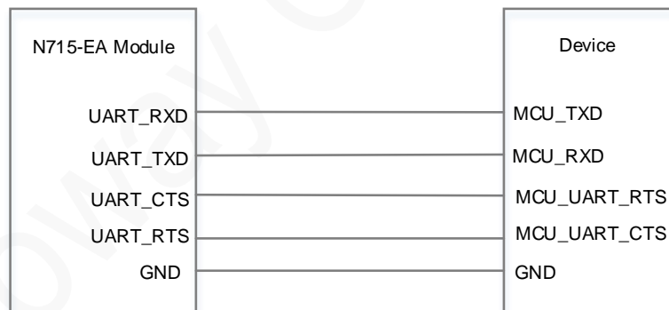
Figure 5-15 Reference design of UART interface
