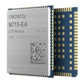
N715-EA is Neoway 2nd-Generation LTE Cat.1 module that support 2G feature. Which would be much suitable for the smart meter and further sharing product. It Adopts the 3GPP Rel.13 LTE technology, which could deliver 10Mbps downlink and 5Mbps uplink data rates.
