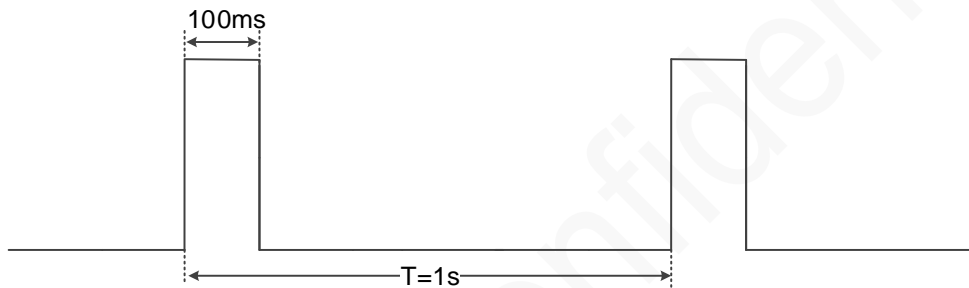
Figure 5-38 Schematic diagram of 1PPS output waveform
