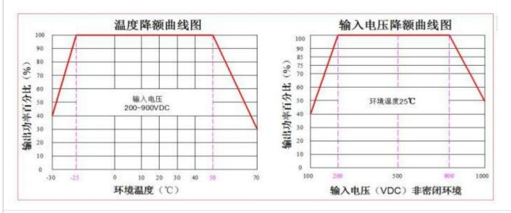
Note 1: When the input voltage is 100~1000VDC and the temperature is -30~70 °C, the voltage derating needs to be performed on the basis of the input voltage derating curve.
